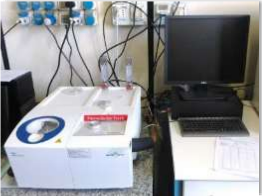
Mettler DSC 1: melting enthalpy and specific heat measurements for PCMs
