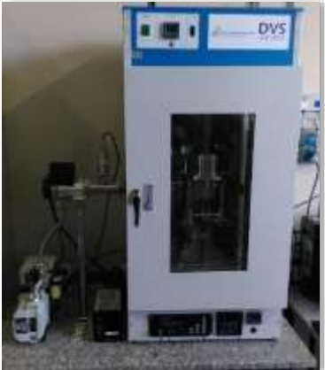
DVS Vacuum: absorption / co-absorption of vapour on solids and liquids
