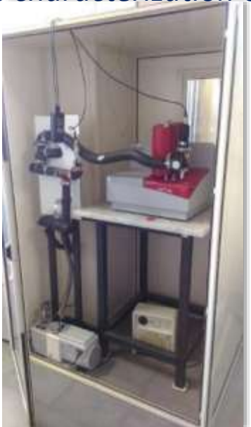
Labsys Evo: TG/DSC under saturated vapour pressure conditions
