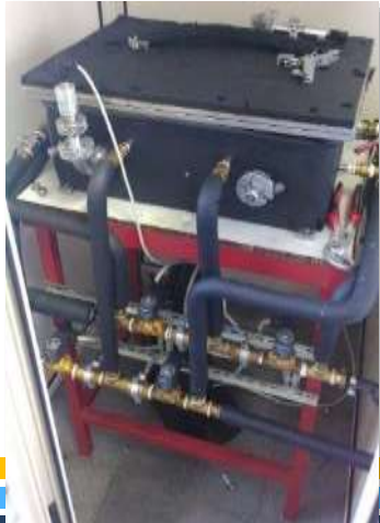
Hydrothermal ageing of sorbent materials under real working boundaries
